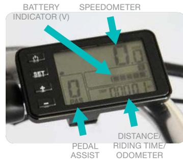
Your Pedego is equipped with an LCD meter that monitors pedal assist, speed, odometer, trip distance, riding time, and battery energy level. To turn the meter on, make sure the battery is fully inserted into the Pedego and the on/off switch is in the on “|” position.
