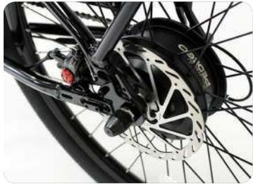
Your Pedego is equipped with disc brakes for maximum reliability. Applying hand pressure to the brake levers will cause the wheel brake to cause friction against the brake disc, slowing the wheel. The more hand pressure applied to the brake lever, the faster the Pedego will come to a stop.
