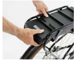
To be able to use the electric motor, the battery must be mounted by sliding the fully charged battery forward into the battery holder.
