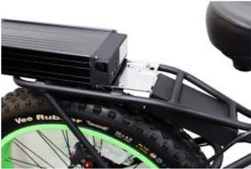
To be able to use the electric motor, the battery must be mounted by sliding the fully charged battery forward onto the rear rack, over the rear wheel, through the channels on the battery while the carry handle is positioned at the rear. The key switch position must be in the “unlock” position to slide the battery on.
