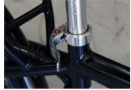
If necessary, tighten the clamp by twisting the clamp handle clockwise while in the unclamped position. Then, fold the handle in toward the seat post. This should require a fair amount of force to ensure the seat post is held tight. If necessary, the clamp can be further tightened with a 5 mm allen wrench while in the clamped position. Make sure the seat is not set with the vertical maximum height marks above the clamp.
