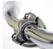
If need be, the angle of the handlebars may be positioned to your personal preference. Loosen the front 2 bolts on the front stem plate and angle the handlebars to your liking, then securely tighten the 2 bolts on the front stem plate. Make sure that, when tightening, there is even spacing between the top and bottom bolts to ensure maximum stability.
