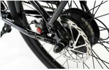
Your Pedego is equipped with disc brakes for maximum reliability. Applying hand pressure to the brake levers will cause the wheel brake to cause friction against the brake disc, slowing the wheel. The more hand pressure applied to the brake lever, the faster the Pedego will come to a stop. The rear brake should always
