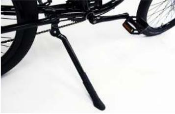
The “side stand” style kickstand has a single leg that flips out to one side and allows the bike to lean against it.
